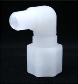
1/4" NPT X 1/4" Tube X 90° Kynar Fitting
